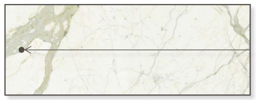
When cutting a "U" shaped piece, mark, and drill relief holes where the cut lines intersect. Always make the shortest cut first.
